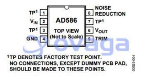
Figure 4. Pin Configuration (R-8)
